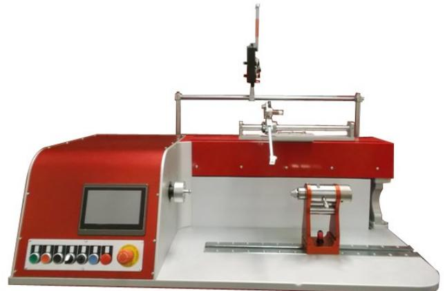
This machine is designed for the manufacture of solenoids, inductors and transformers, (with capacity to make multiple windings), and small distribution and power transformers.
