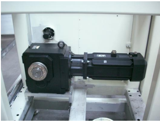
The system incorporates high torque Parker servo motors with integrated reduction drive systems for precision control.
