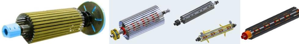
As can be seen in the photos, the expanding mandrel are finished with aluminium bars and wood mounted on the outer diameter. Each mandrel has a built in gearbox which is driven by a pneumatic hand tool, which expands the mandrel for winding and then collapses it for easy removal of the coil at the end of the winding process. Larger versions can be provided with an expanding and contracting mechanism that is powered by hydraulics.
