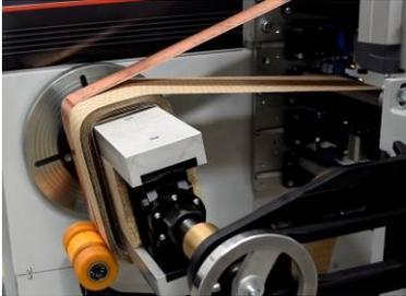
The new generation of expandable mandrels provide the possibility of winding with rectangular, circular or ovoid shape coils, without changing mandrel.
