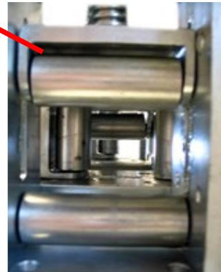
The reason for this is to bring multiple wires coming from different supply spools together - forming a single packet to then wind onto the core / bobbin.
