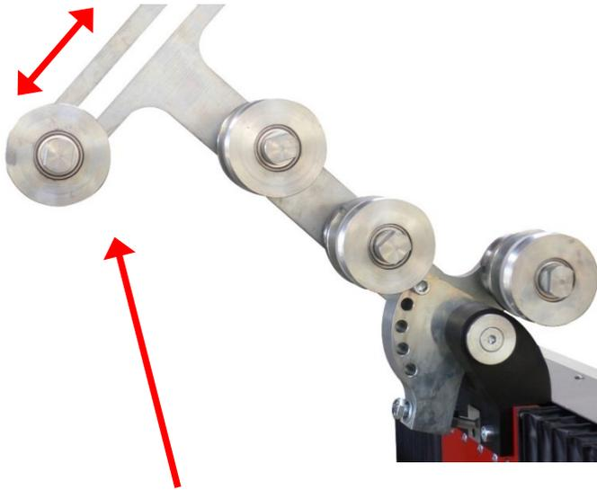
The front roller is also adjustable in height / angle. This "negative effect" roller can be used to produce an upward curve on the wire. When wound onto the flat sides of the bobbin the inverse curve of wire presses against the long flat edges of the bobbin, reducing the bow effect
