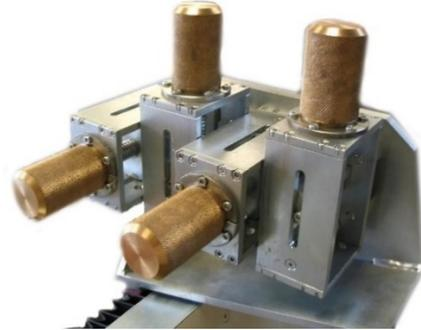
This guide has at the rear, a series of four parallel roller sets, each is mounted at 90° to the previous one and independently adjustable.
