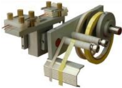
Multi-wire feeder head with margin taping
