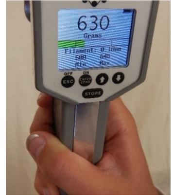
Large, easy to read backlit, graphic display with adjustable backlighting and contrast. Data Logging feature included; Capture and view data within a user-defined time window. Select the time window; then select the sampling rate (from 1-100 Hz).
