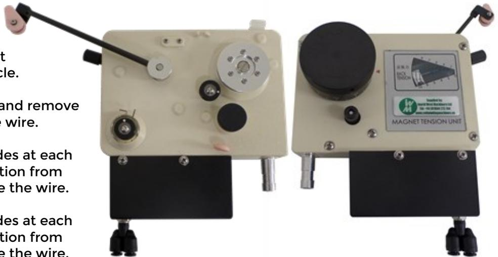
The models shown have a pneumatic cylinder (controllable from the winding machine) for tension release as required during pin wrapping operations as well as microswitch detecting arm moving up indicating wire brake.
