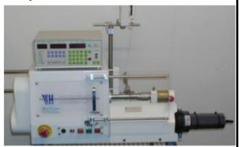
Precise control of the heat-gun air temperature and air flow rate, and exact positioning of the nozzle, warm the wire and the tooling just enough to guarantee perfect bonding of wire to wire, whilst releasing from the tool at the end of the cycle.
