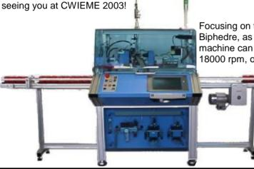
Focusing on the high-precision workings of a GS-Automation Biphedre, as shown at CWIEME 2002. This free-standing automatic machine can wind wire from 0.01 mm to 1 mm in diameter, at up to 18000 rpm, onto cores from 0.3 mm to 80 mm in diameter.
