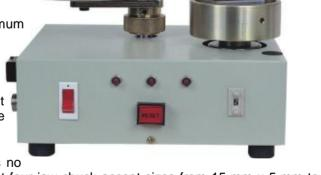
It has a foot switch for optimum productivity, and there is no special tooling required for each bobbin as the independent four jaw chuck accept sizes from 15 mm x 5 mm to 63 mm x 63 mm and uses Magnetic pads (mounted on the jaws) allowing the operator to simply drop in the core... fast operation (Max speed 90 rpm)
