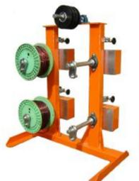
To avoid damage to the insulation when tensioning thick wire, tension must be applied to the supply spool. Our range of 1, 2, 4 & 32 spindle tension units use hydraulic callipers to accurately control the force applied.
