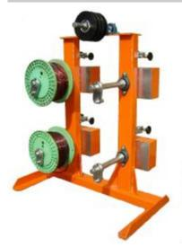
To avoid damage to the insulation when tensioning thick wire, tension must be applied to the supply spool. Our range of 1, 2, 4 & 32 spindle tension units use hydraulic callipers to accurately control the force applied.
