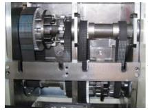
4-ratio quick change spindle drive provides maximum versatility for fast primary winding at high speed, whilst smoothly delivering the necessary torque at lower speeds. The EZ-900 is capable of pulling the heaviest of wires.
