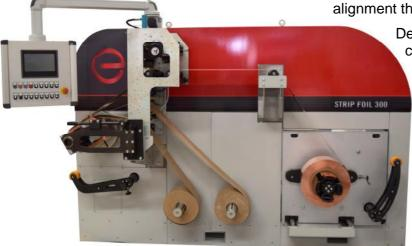
Design flexibility provides for various combinations of conductors, interleaved insulation and edge fillers, together with a choice of cold pressure or TIG welding of terminals.
