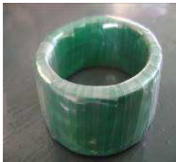
The finished taped core
