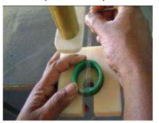
With the help of "Air Jet", the tape will be pushed through the core, after that, we have to bring the tape over the top of the toroid to produce the wound tape turns...
