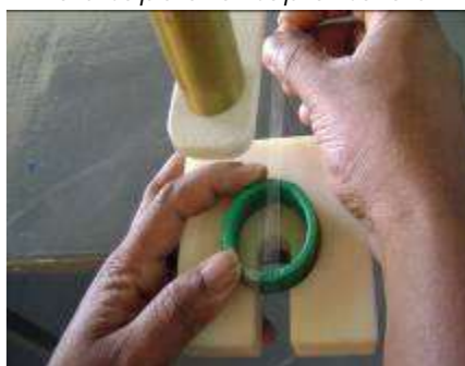
Hold tape over top of toroid
