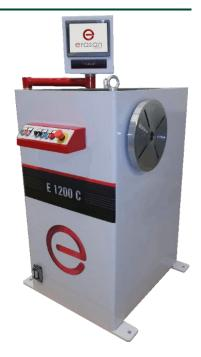
This machine is specially designed for the manufacture of solenoids and power and distribution transformers from 10 to 1.200 KVA, using aluminium or copper wires, including rectangular or flat wires.
