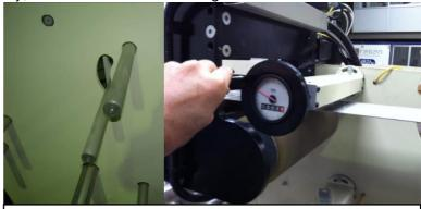
Each mandrels foil or insulation has independent traversing system, with feedback from edge sensor, providing perfectly aligned coils
