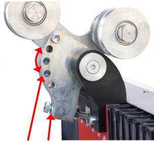
The guide head angle is adjustable; Course adjustment in steps of 18° Fine adjustment from bolt underneath
