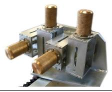
This guide has at the rear, a series of four parallel roller sets, each is mounted at 90° to the previous one and independently adjustable.
