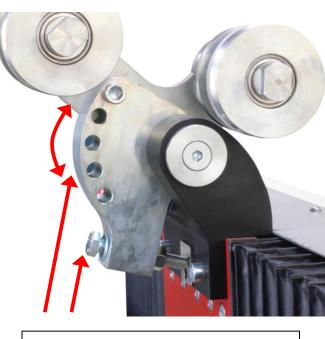
The guide head angle is adjustable; Course adjustment in steps of 18° Fine adjustment from bolt underneath
