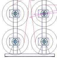
The front section of the quider head has two profile rollers, adjustable width & Teflon side walls to protect the wire insulation.
