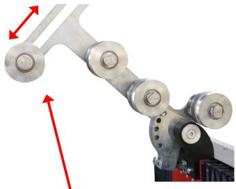
The front roller is also adjustable in height / angle. This "negative effect" roller can be used to produce an upward curve on the wire.
