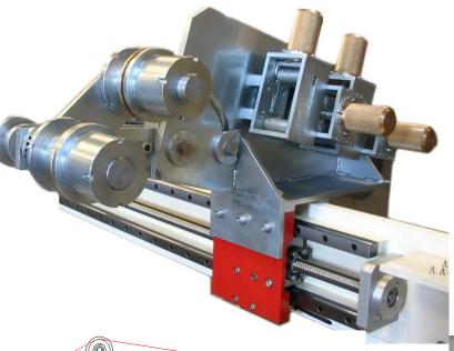
This guide has at the rear, a series of four parallel roller sets, each is mounted at  $90^{\circ}$  to the previous one and independently adjustable.
