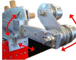
The front roller is also adjustable in angle. This "negative effect" roller can be used to produce an upward curve on the wire, meaning when wound onto flat sides of bobbin, the inverse curve of wire presses against the long flat edges, reducing the bow effect
