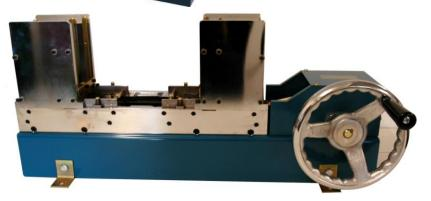
Laminations of 0.35 mm to 0.5 mm thick are stacked at up to 300 pieces per minute, manually or automatically, with full interleaving.
