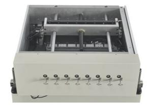
When making a solder connection to fine wire, the mechanical strength of a single strand of wire may not be sufficient. The skeining unit reinforces the start and finish leads of the winding by twisting multiple strands of the wire together, so that they can withstand the soldering process.
