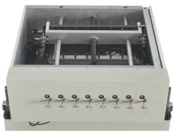
When making a solder connection to fine wire, the mechanical strength of a single strand of wire may not be sufficient. The skeining unit reinforces the start and finish leads of the winding by twisting multiple strands of the wire together, so that they will then withstand the soldering process.
