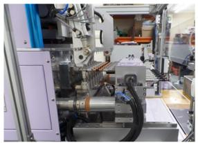
Allows automated load and unload, improving the machine throughput/cycle, and allowing easy access for extra stations to be added to the line, e.g soldering, welding etc.
