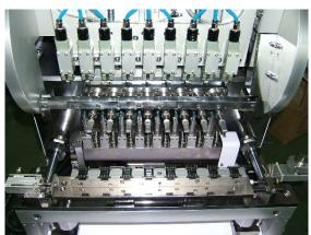
For cutting larger wire diameters the pin tear method will no longer work. In this case we can fit air operated cutters close to the nozzle head.
