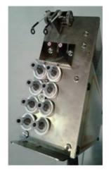
Integral Disc Tensioner with easy thread discs
