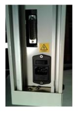
Serial Link connection. Easily interfaced with most winders
