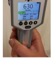
Large, easy to read backlit, graphic display with adjustable backlighting and contrast. Data Logging feature included; Capture and view data within a user-defined time window. Select the time window, then select
