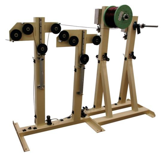
The tensioning device provides wire tension by applying a braking force to the wire spool, eliminating the possibility of causing damage to the wire insulation.
