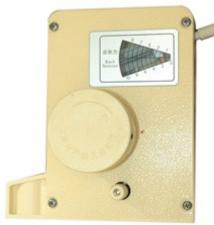
The arm position provides feedback to the system, adjusting the main friction wheel to regulate and maintain constant tension during the winding cycle.
