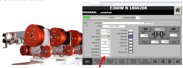
Tension setting, Set from within each step of the winding cycle, and stored directly with the winding program.
