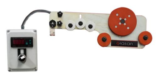
The supply voltage is 230V single phase and the maximum power consumption is 25W.
