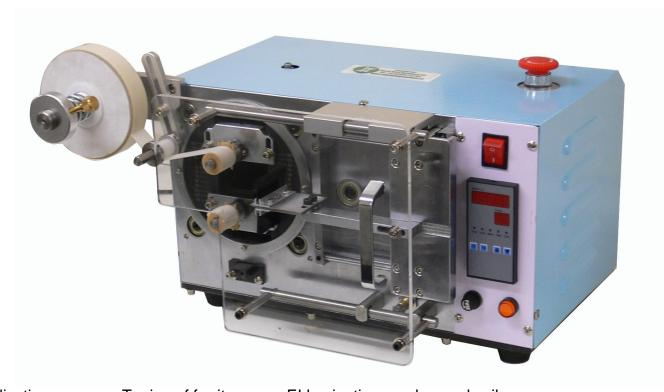
Application: Taping of ferrite cores, EI laminations and wound coils.
